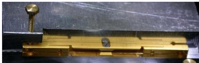
Figure 2. Taper glued on the holder.
